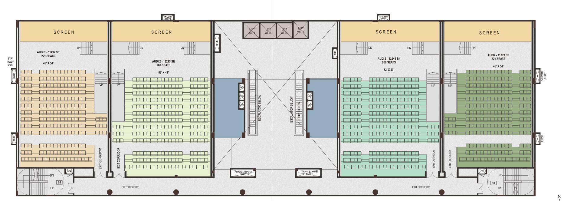
Box office area is provided in the Ground floor. Projector room, Server room & back office are provided in upper level. Concession areas & Toilets are at Audi entry level.
